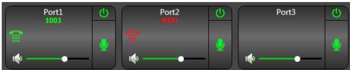
Figure 5-15: An interface that is successfully registered to a SIP account (left), one that has had incorrect registration credentials provided (middle), and one that is not associated with a SIP account (right).
