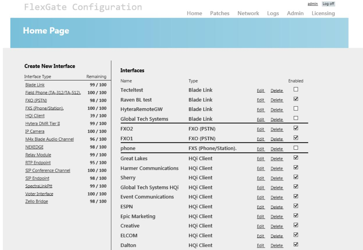
Figure 2-1: Home screen for the FlexGate web configuration tool. The left side displays the different interfaces that are available. The right side of the screen displays the interfaces that have already been created.
