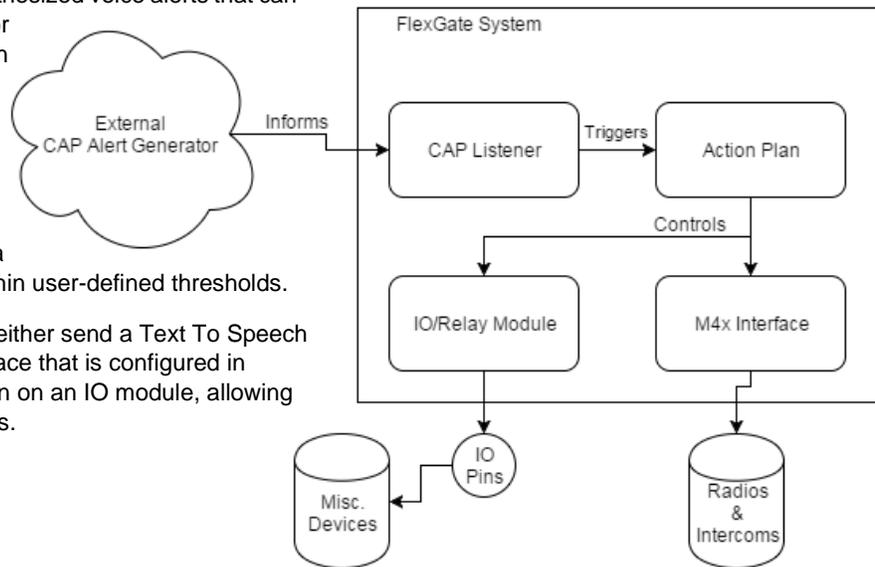
Figure 6-1: The architecture of the Action Plan workflow.
