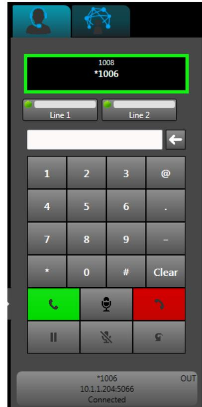
Figure 5-4: The SIP phone control. This dial pad is used to manage SIP and traditional phone line calls.
