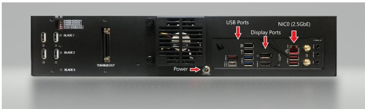
Figure 1-1: FlexGate Back Plane Diagram
