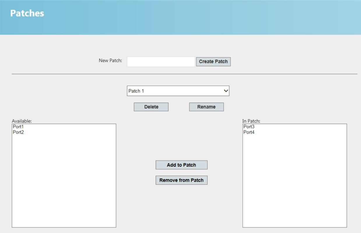
Figure 3-1: The Patches page from the configuration website. Here you can create, delete, and reconfigure your FlexGate communication patches.
