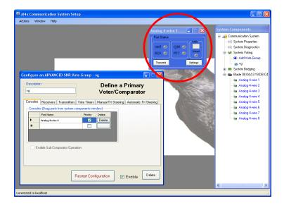
Similarly, the "Configure An Advanced SNR Vote Group" window (shown circled below) should be closed when any changes are being made to a port setting using the "Analog 4-Wire 1" configuration window.
