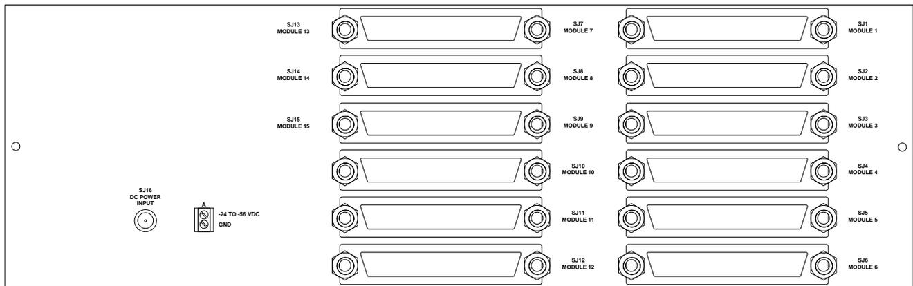
41000-224 Bridge/Hybrid/Notch Filter Shelf with Redundant Power Supplies
